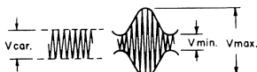
Fig.4 - The amplitude modulated wave; V_{car} is the amplitude of carrier before modulation.
